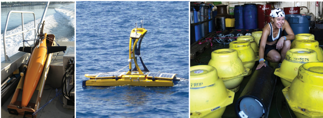
FIGURE 9. (left) Ocean glider. Courtesy of LADC-GEMM. (center) Autonomous surface vehicle. Courtesy of ASV Global. (right) Moored hydrophone (black cylinder) with line of buoys. Courtesy of LADC-GEMM
