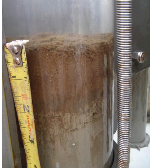
FIGURE 9. A thick, fluffy floc layer sampled from the seafloor, as observed in a sediment core taken in the Gulf of Mexico. Photo taken in September 2010. Courtesy of ECOGIG/Samantha Joye
